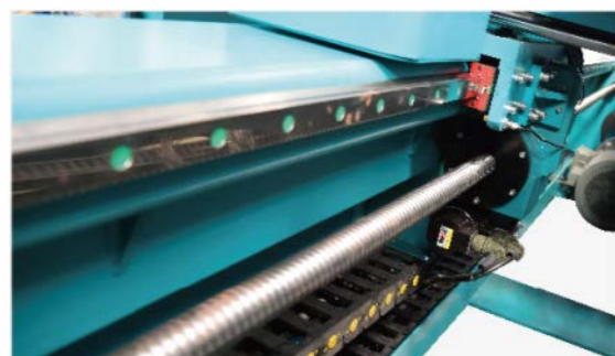
▲ 导轨排布：二条高精度直线导轨，分布在撑挡内外二侧面 Guide rail: Two high-precision linear guide rails, installed on each side of the wall
