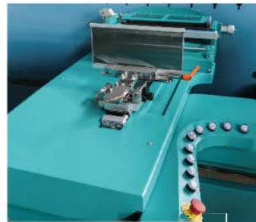
▲ 整经台：具有测力和测密功能的整经台 Warping table: With function of tension and density measurement
