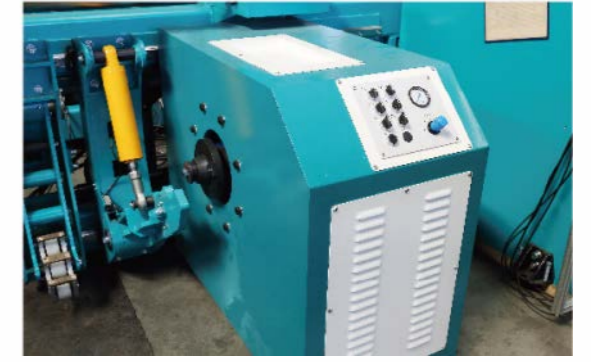
▲ 拍开拍合：齿轮箱左右移动实现拍开拍合 Clap/unclap: Achieved by gearbox moving leftward & rightward
