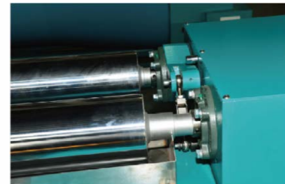
▲ 上油上蜡装置：倒轴时上蜡可以改善某些纱线在织造过程中的运行性能。可以对上蜡进行任意编程控制，从而确保上蜡均匀。 Oiling/waxing device: For better working performance in weaving process of some kind of yarn. Programme controlled to ensure uniform waxing.
