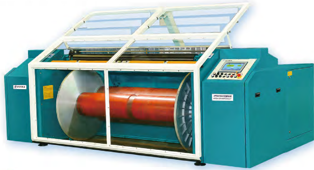
染色经轴整经 Dyeing beam warping
