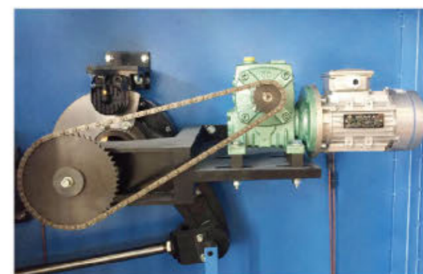
压辊左右微调装置 Fine adjust device on right and left side of press roller 通过减速电机可调整压辊与经轴盘片之间的距离 Distance between press roller and beam flange can be adjusted by gear motor
