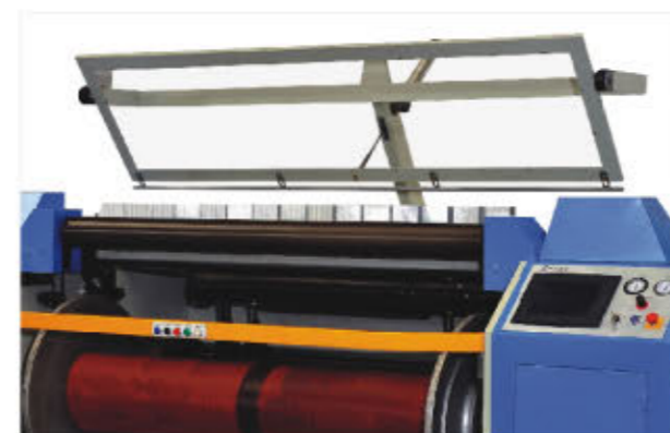
简易挡风罩 Simple windshield 通过气缸推拉，控制挡风罩升降 Lifting of windshield is controlled by cylinder
