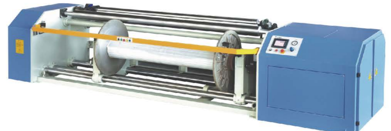
▲ 上油上蜡装置：通过无级变速器调整上油辊转速，从而上油量与倒轴线速度恒定。 Oiling/waxing device: Oiling roller speed is adjusted by step-less speed-transmission, achieve oiling amount and beaming linear speed to be constant.
